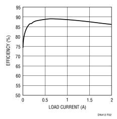
Figure 2. The LT3681 Boasts High Efficiency (12V Input to 5V Output)
